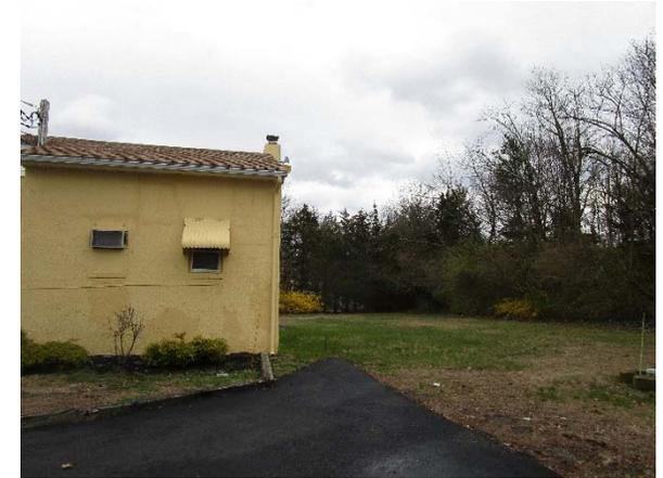
A rain garden can be installed in the turfgrass area on the south side of the building to capture, treat, and infiltrate stormwater runoff from the roof. A preliminary soil assessment suggests that the soils have suitable drainage characteristics for green infrastructure.
