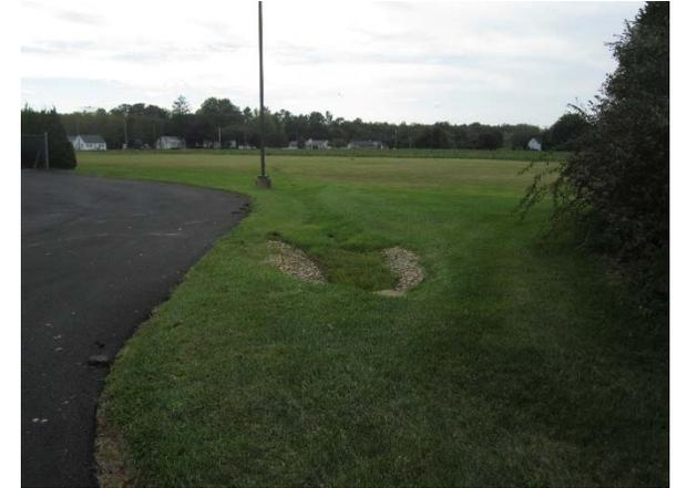
A rain garden can be installed on the west side of the property to capture, treat, and infiltrate stormwater runoff from the parking lot and to enhance a currently existing drainage area. A preliminary soil assessment suggests that the soils have suitable drainage characteristics for green infrastructure.
