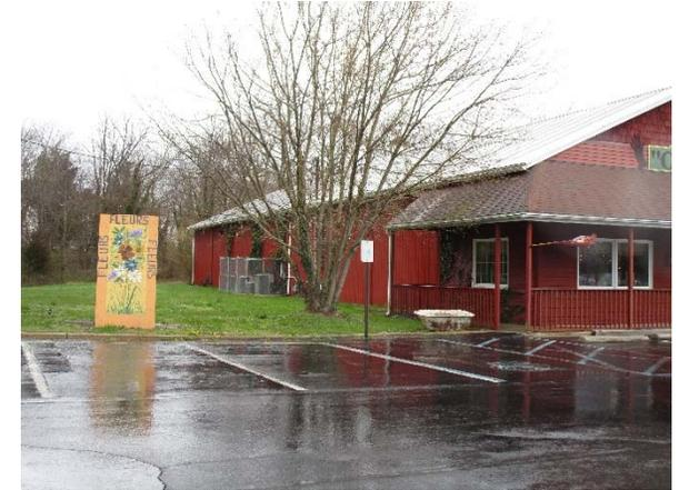
A rain garden can be installed in the turfgrass area on the west side of the building to capture, treat, and infiltrate stormwater runoff from the roof. The downspout at the southeast corner of the building can be connected to a downspout planter box to allow rooftop runoff to be filtered and reused. A preliminary soil assessment suggests that more soil testing would be required before determining the soil's suitability for green infrastructure.
