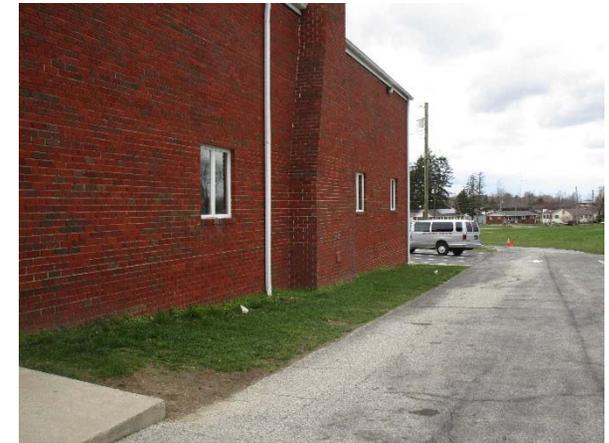
A section of parking spaces can be replaced with pervious pavement to capture and infiltrate stormwater runoff from the parking lot. Rain gardens can be installed in the turfgrass around the property to capture, treat, and infiltrate stormwater runoff from the roof of the building and the parking lot. A preliminary soil assessment suggests that the soils have suitable drainage characteristics for green infrastructure.
